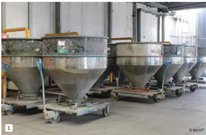
**1** The tubs are metal containers used for the powder coatings in different production stages.
