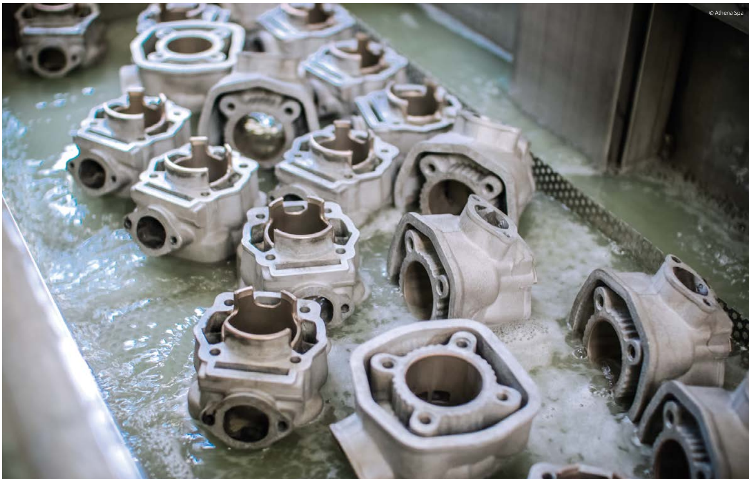
The cleaning phases before and after the galvanic process are essential for the final quality of components.
